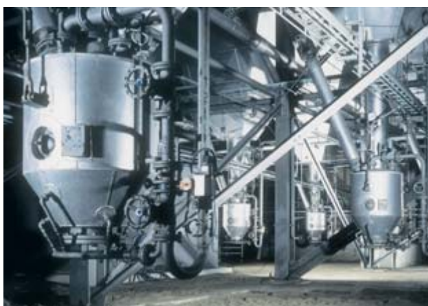
Pressure vessel ash collecting system
